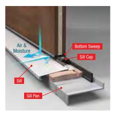
Sill and bottom sweep form a tight seal against wind-driven moisture infiltration at the bottom of the door system and help channel moisture away from the home. Sill pan (recommended) adds an extra layer of protection to help keep moisture away from the subfloor.
